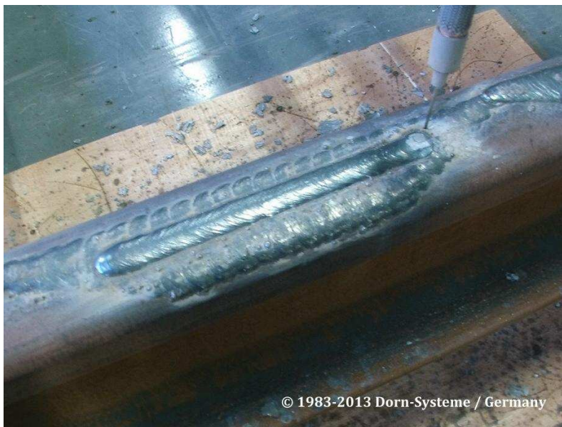
Line-Mode welding with constant movement and small size, fast oscillation
